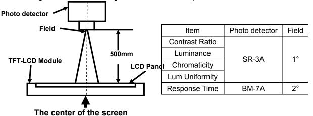
Note 2: Definition of viewing angle range and measurement system. viewing angle is measured at the center point of the LCD by CONOSCOPE(ergo-80).
