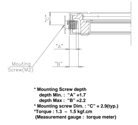
Notes : 1. Screw plated through the method of non-electrolytic nickel plating is preferred to reduce possibility that results in vertical and/or horizontal line defect due to the conductive particles from screw surface.
