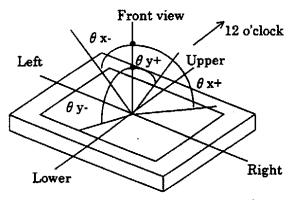
note 4: Viewing angle is  $\theta x = \pm 0^{\circ}$ ,  $\theta y = \pm 0^{\circ}$ . At center.
