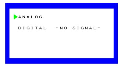
2. NO SIGNAL: "NO SIGNAL" is displayed for four seconds when signals are no input.
