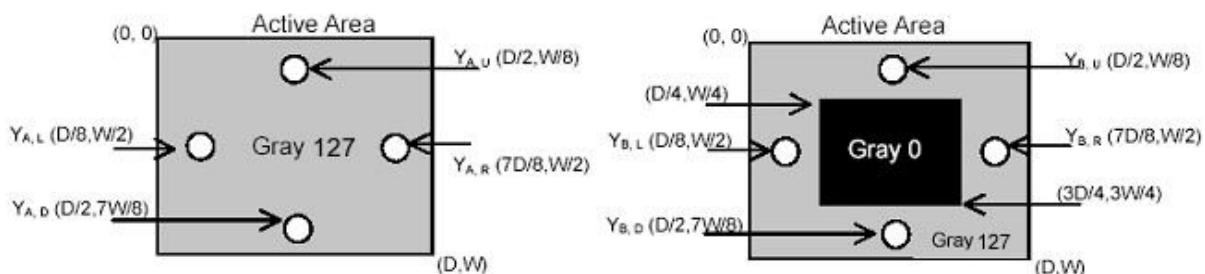
**Note 9: Test Pattern: Subchecker Pattern measured by TOPCON SR-3**
