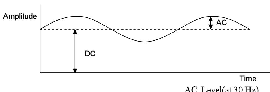
$$\text{Flicker (dB)} = 20 \log \frac{\text{AC Level(at 30 Hz)}}{\text{DC Level}}$$
