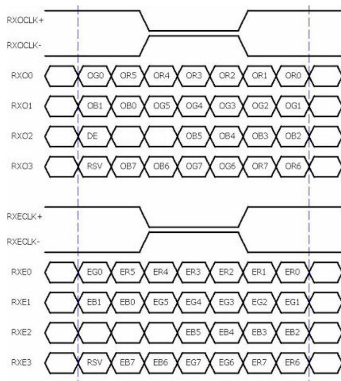
**Note 1:** R/G/B data 7:MSB, R/G/B data 0:LSB    O = "First Pixel Data"    E = "Second Pixel Data"
