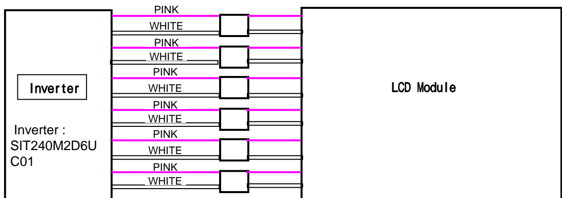
Fig. Measurement point of Lamp Current
