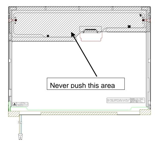
Note 1) Never push this area. Pushing here may cause the LCD being damaged.
