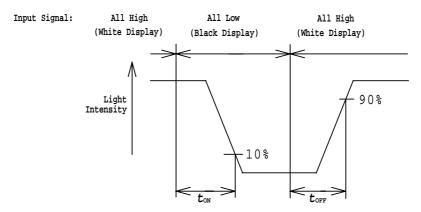
$t_{\rm ON}$ : Turn on time is the time for a photo detector output waveform to go from maximum value to 10% of its maximum.  $t_{\rm OFF}$ : Turn off time is the time for a photo detector output waveform to go from zero to 90% of its maximum.
