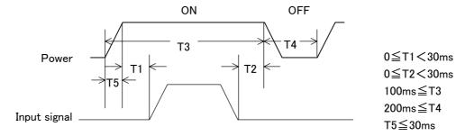
note…The time regulations from T1 to T5 are defined as a changing point 10% of the amplitude of "Input signal" and "Power", and 90%.
