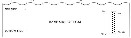
The backlight interface connector is a model BHR-03VS-1, manufactured by JST. The mating connector part number is SM02(8.0)B-BHS-1-TB or equivalent. The pin configuration for the connector is shown in the table below.
