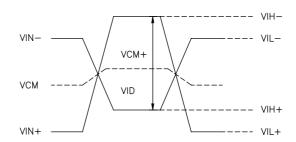
VIN+ : Positive differential DATA & CLK Input VIN- : Negative differential DATA & CLK Input (2) Backlight \*1)
