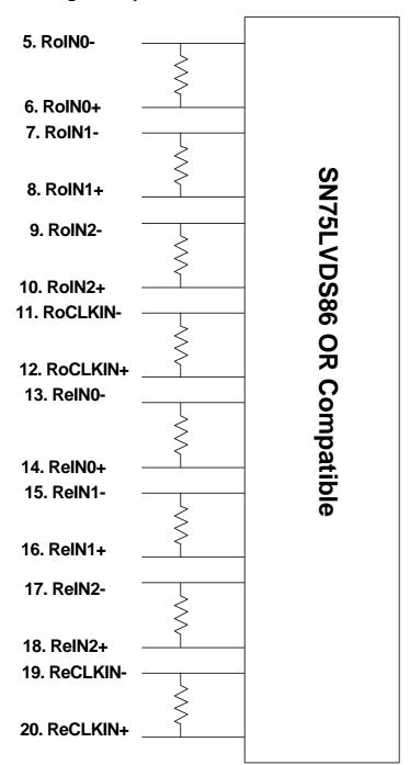
The module uses a 100ohm resistor between positive and negative data lines of each receiver input
