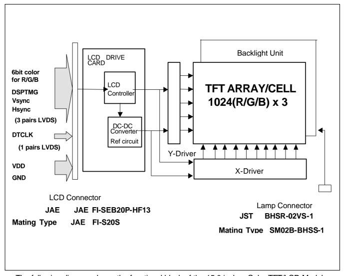
The following diagram shows the functional block of the 15.0 inches Color TFT/LCD Module:
