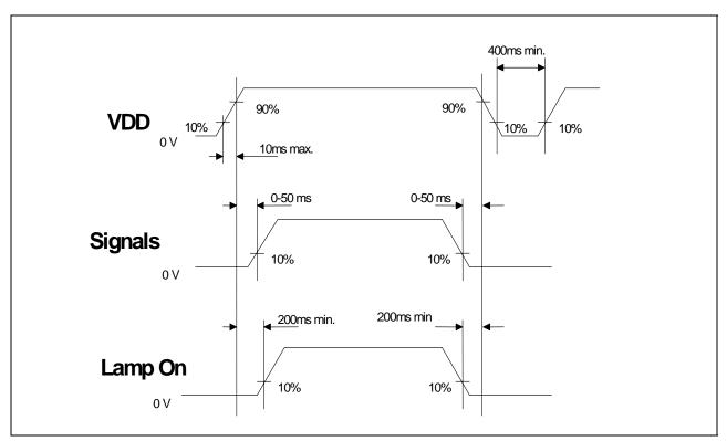
VDD power and lamp on/off sequence is as follows. Interface signals are also shown in the chart. Signals from any system shall be Hi-Z state or low level when VDD is off.
