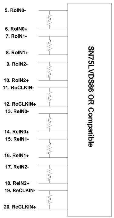
The module uses a 100ohm resistor between positive and negative data lines of each receiver input
